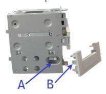
Figure 4 - 15 : Removing the Plastic Kit
